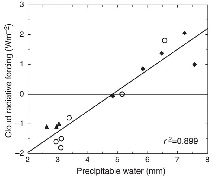
**Figure 7.3:** Relationship between simulated global annually averaged variation of net cloud radiative forcing at the top of the atmosphere and precipitable water due to CO<sub>2</sub> doubling produced in simulations with different parametrizations of cloud related processes. Results are from Colman and McAvaney (1995) denoted by triangles, Meleshko *et al.* (2000) denoted by open circles, and Yao and Del Genio (1999) denoted by diamonds.
