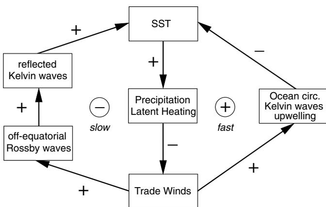
**Figure 7.8:** Simplified principal feedback loops active in El Niño-Southern Oscillation (ENSO). The fast loop (right) gives rise to an instability responsible for the development of an El Niño, the slow loop (left) tends to dampen and reverse the anomalies, so that together, these processes excite oscillations.
