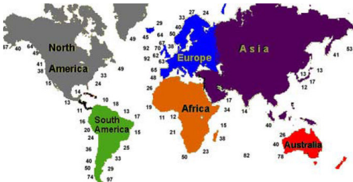
Figure 4.3.13: Annual average wave power flux (kW/m) across the oceans (Wavegen, 2004).
