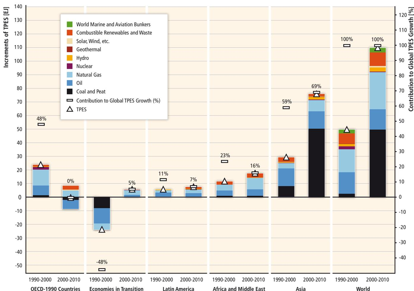
**Figure 7.2** | Contribution of energy sources to global and regional primary energy use increments. Notes: Modern biomass contributes 40% of the total biomass share. Underlying data from IEA (2012a) for this figure have been converted using the direct equivalent method of accounting for primary energy (see Annex.II.4). Legend: OECD-1990 (OECD-1990), Asia (ASIA), Economies in Transition (EIT), Middle East and Africa (MAF), and Latin America (LAM), total primary energy supply (TPES).
