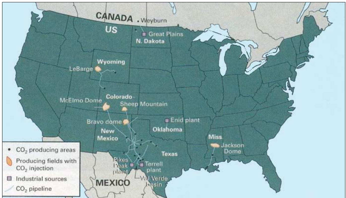
Figure 4.1 CO 2 pipelines in North America. (Courtesy of Oil and Gas Journal).
