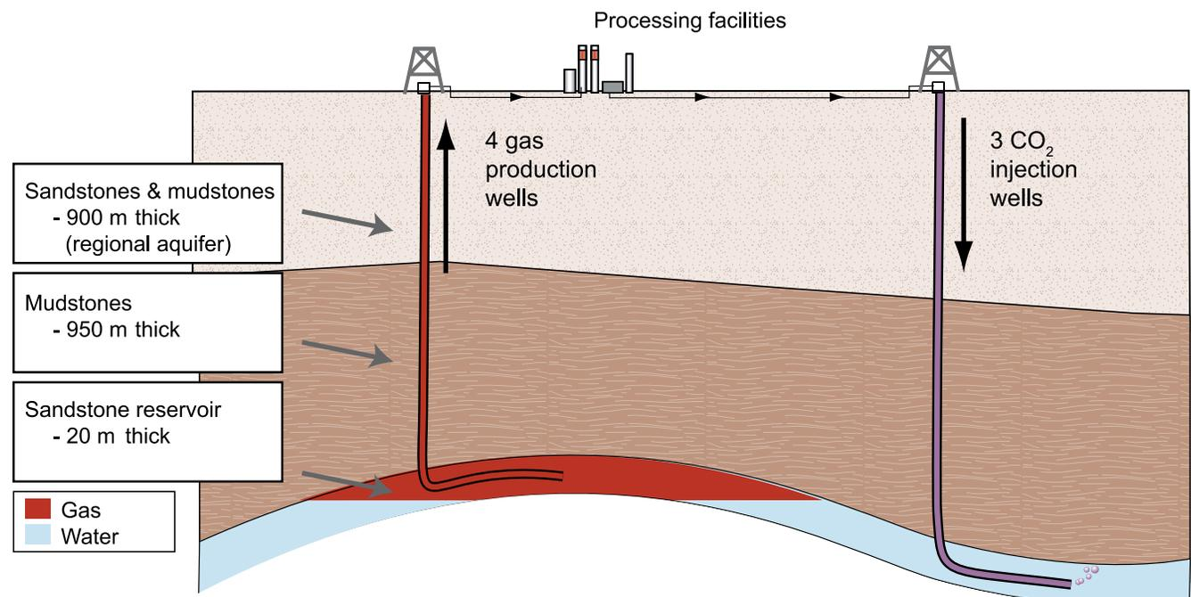
**Figure 5.5** Schematic of the In Salah Gas Project, Algeria. One MtCO<sub>2</sub> will be stored annually in the gas reservoir. Long-reach horizontal wells with slotted intervals of up to 1.5 km are used to inject CO<sub>2</sub> into the water-filled parts of the gas reservoir.
