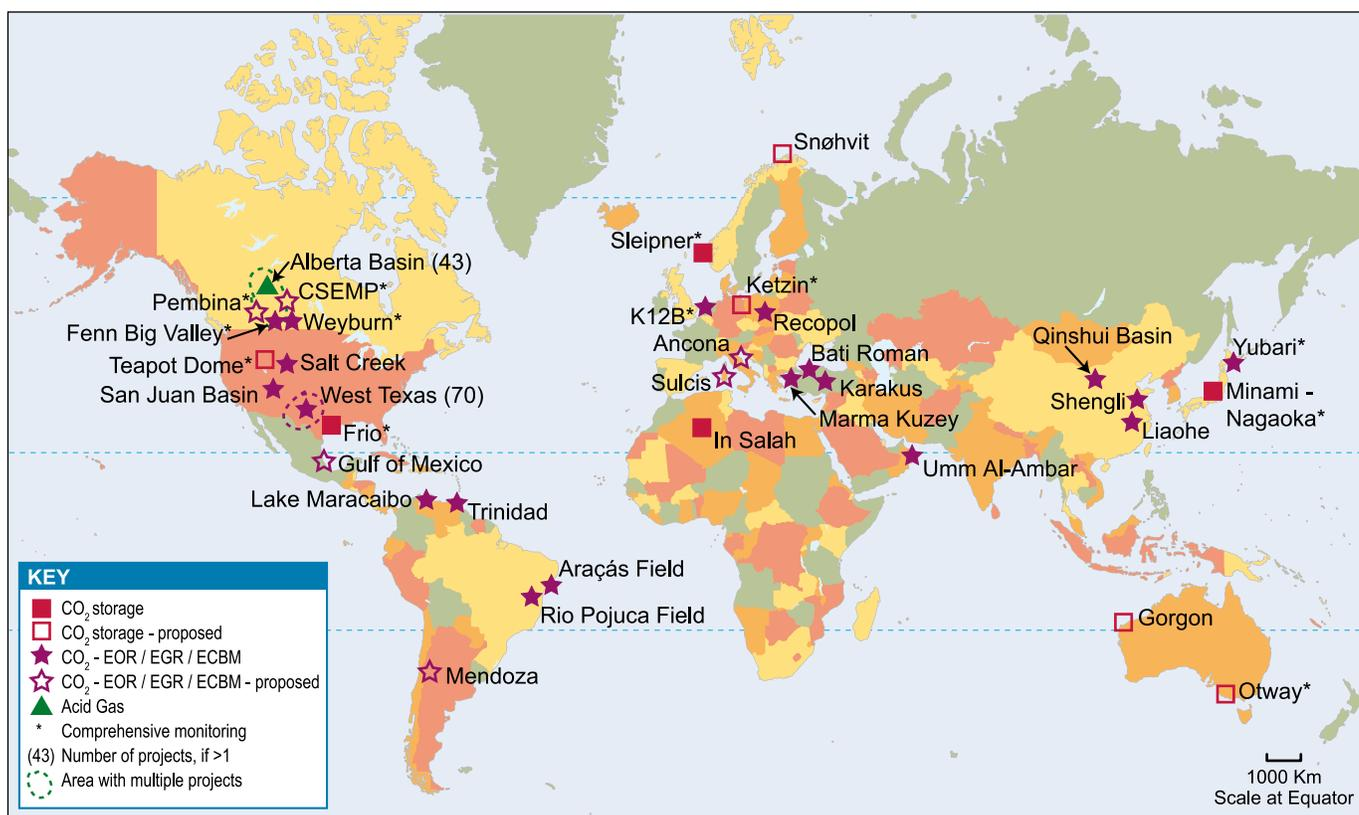
**Figure 5.1** Location of sites where activities relevant to CO<sub>2</sub> storage are planned or under way.
