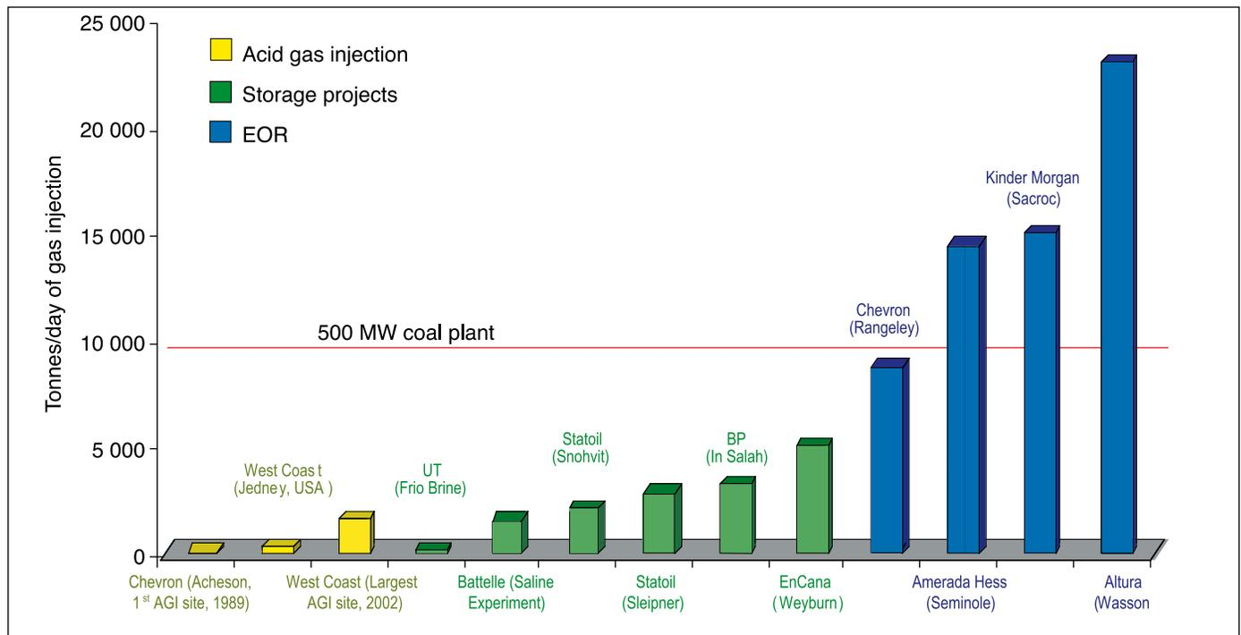
**Figure 5.22** Comparison of the magnitude of CO<sub>2</sub> injection activities illustrating that the storage operations from a typical 500-MW coal plant will be the same order of magnitude as existing CO<sub>2</sub> injection operations (after Heinrich *et al.*, 2003).
