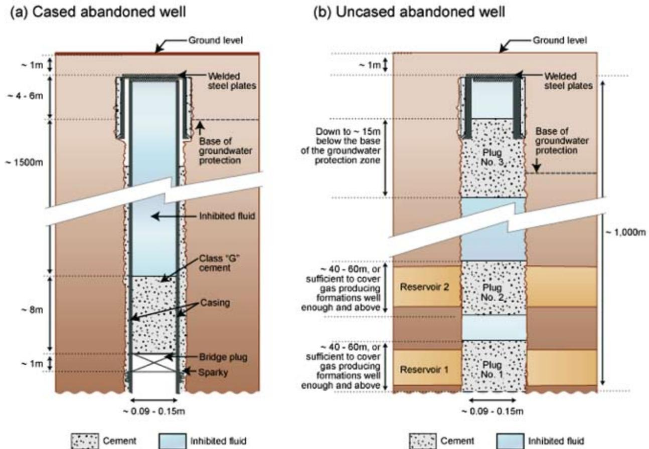
**Figure 5.21** Examples of how cased and uncased wells are abandoned today. Special requirements may be developed for abandoning CO<sub>2</sub> storage wells, including use of corrosion-resistant cement plugs and removing all or part of the casing in the injection interval and caprock.
