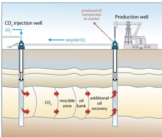
**Figure 5.15** Injection of CO<sub>2</sub> for enhanced oil recovery (EOR) with some storage of retained CO<sub>2</sub> (after IEA Greenhouse Gas R&D Programme). The CO<sub>2</sub> that is produced with the oil is separated and re-injected back into the formation. Recycling of produced CO<sub>2</sub> decreases the amount of CO<sub>2</sub> that must be purchased and avoids emissions to the atmosphere.
