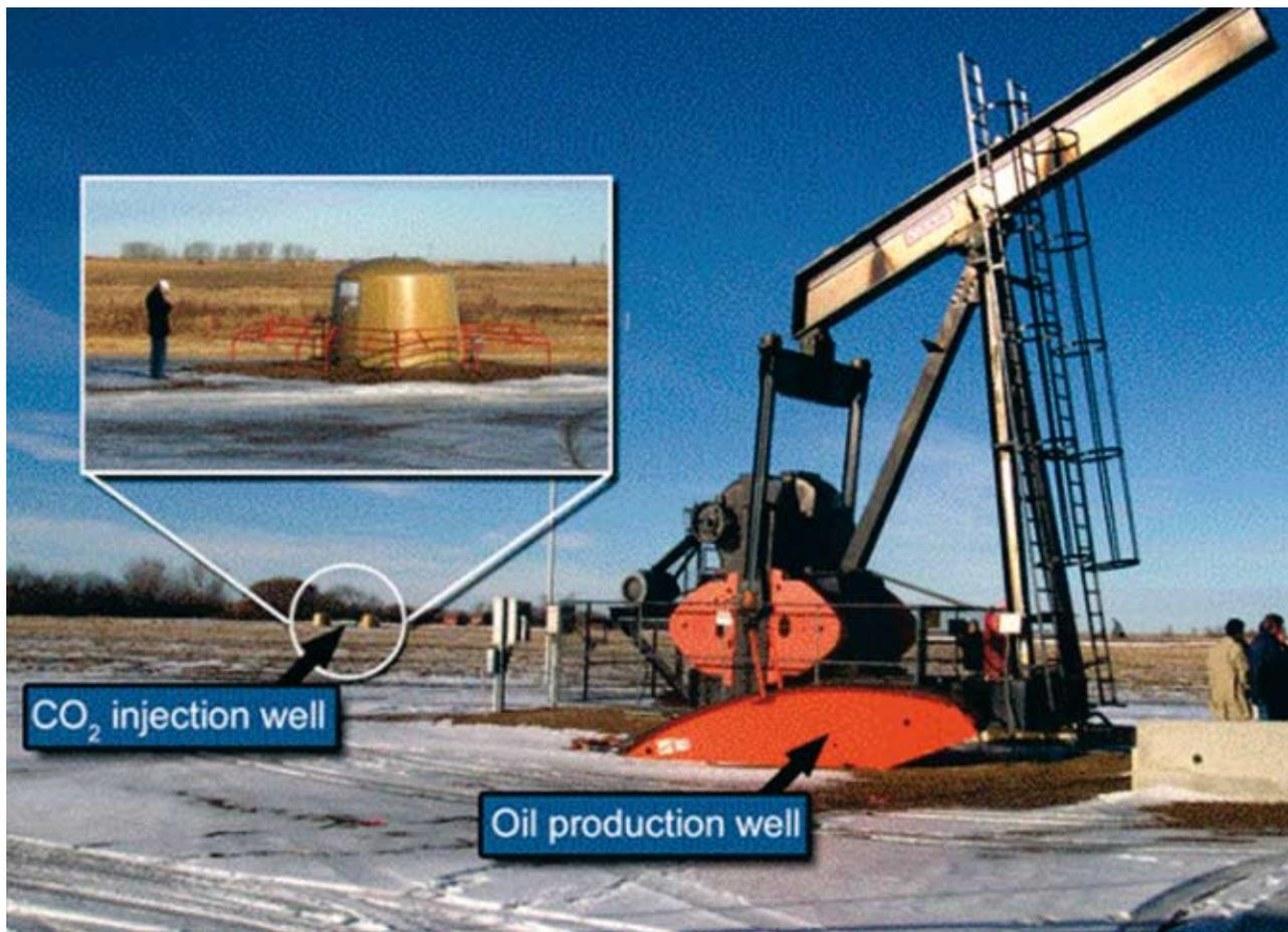
Figure 5.23 Typical CO<sub>2</sub> field operation setup: Weyburn surface facilities.
