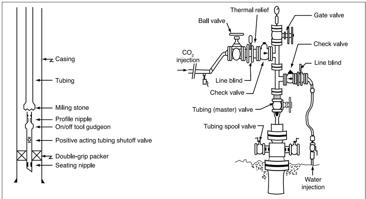
**Figure 5.20** Typical CO<sub>2</sub> injection well and wellhead configuration.
