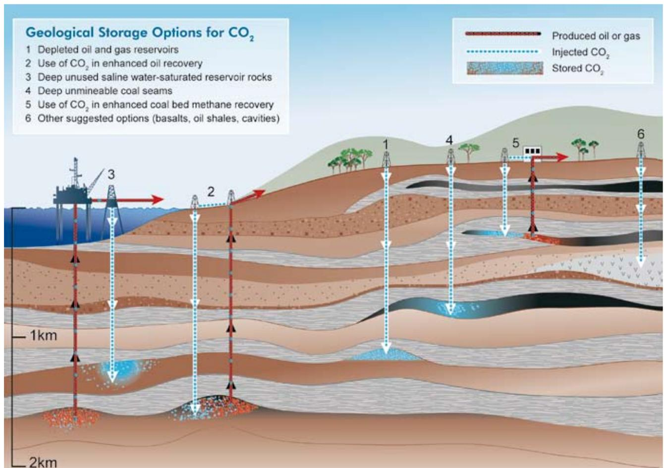
Figure 5.3 Options for storing CO<sub>2</sub> in deep underground geological formations (after Cook, 1999).
