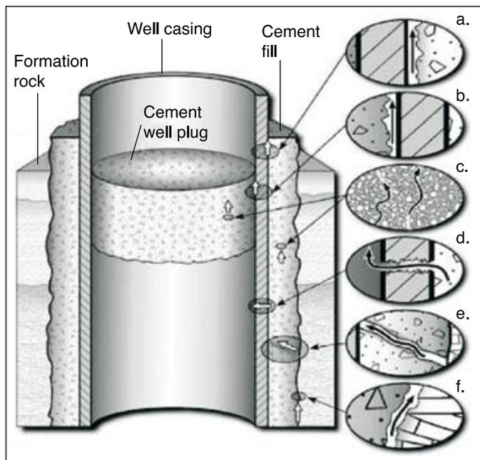
**Figure 5.26** Possible leakage pathways in an abandoned well: (a) and (b) between casing and cement wall and plug, respectively; (c) through cement plugs; (d) through casing; (e) through cement wall; and (f) between the cement wall and rock (after Gasda *et al.*, 2004).
