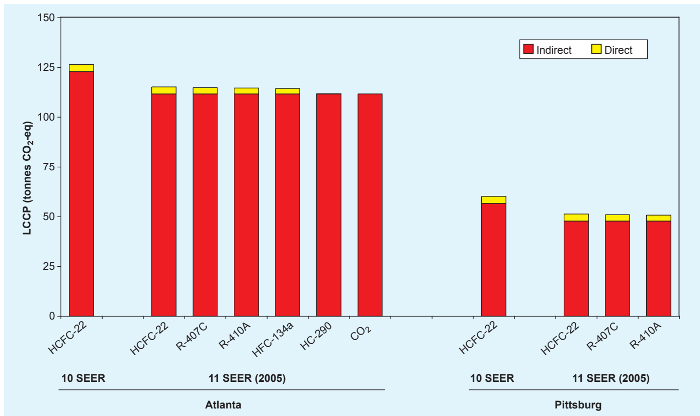
Figure 5.2. LCCP values for a 7.5 tonne (26.3 kW) commercial rooftop air conditioner in Atlanta, Georgia and Pittsburgh, Pennsylvania, USA (ADL, 2002; Sand et al. , 1997).
