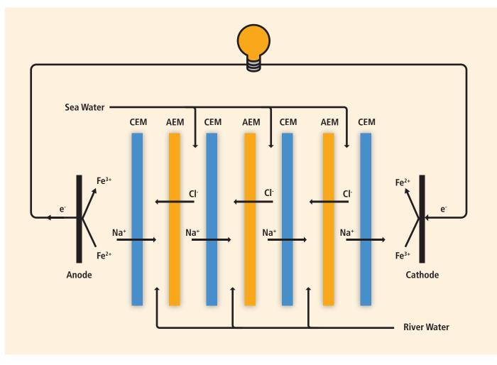
Figure TS.6.4 | Reversed electro dialysis (RED) system. [Figure 6.9]
