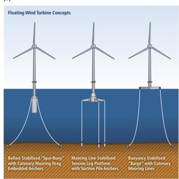
Figure TS.7.4 | Offshore wind turbine foundation designs: (a) near-term concepts and (b) floating offshore turbine concepts. [Figure 7.19]
