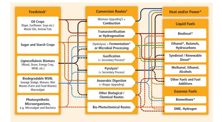
Figure TS.2.3 | Schematic view of the variety of commercial (solid lines) and developing bioenergy routes (dotted lines) from biomass feedstocks through thermochemical, chemical, biochemical and biological conversion routes to heat, power, CHP and liquid or gaseous fuels. Commercial products are marked with an asterisk. [Figure 2.2, 2.1.1]
