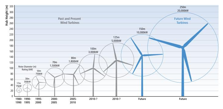
Figure TS.7.2 | Growth in size of typical commercial wind turbines. [Figure 7.6]
