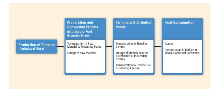
Figure TS.8.5 | The production, blending and distribution system for a range of liquid biofuels is similar regardless of the biomass feedstock. [Figure 8.11]
