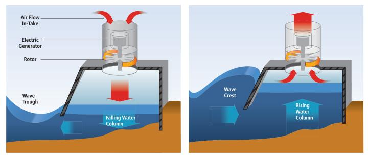
Figure TS.6.2a/b | Type of wave energy converter and its operation: oscillating water column device. [Figure 6.6] (design by the National Renewable Energy Laboratory (NREL))
